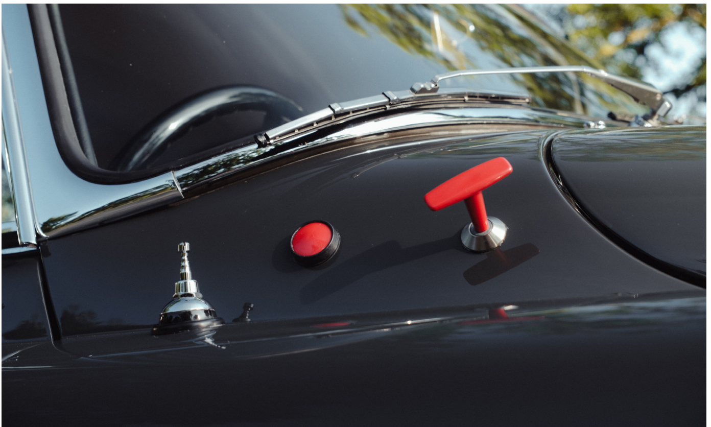
Picture above: Competition fire extinguisher system
