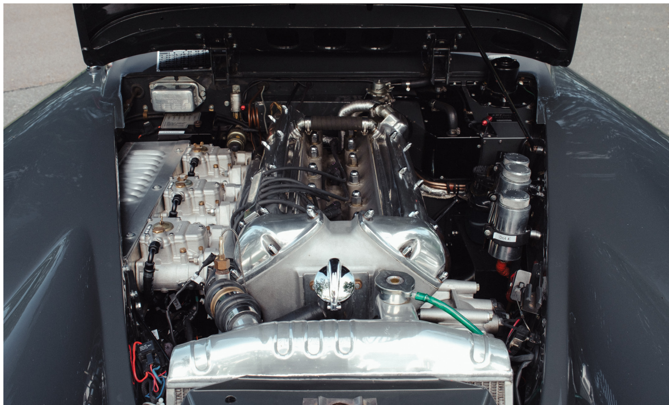
Picture above: 3.8 ltr engine fitted with wide angle D-Type head
